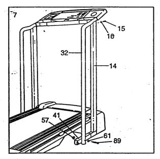
8. Attach the Storage Latch (12) to the left Upright (14) with two 1/2" Screws (13). Be careful not to overtighten the Screws.
